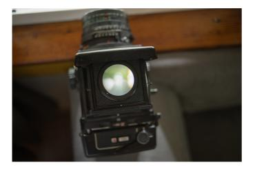
substantially, but framing with a waist-level meter can be quite difficult if you aren't used to it. I almost always use this camera on a tripod, so the inverted image is easier to manage, but if you are handholding this camera it is sometimes really difficult to keep the horizon straight. With practice you can eventually get used to it, but having a prism finder on makes things a lot easier sometimes.
